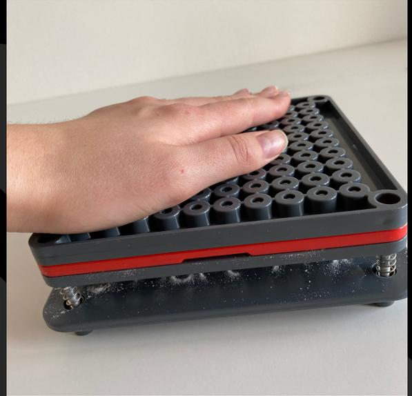
**6.3** Remove the cap plate and the middle plate. Now all the capsules are complete and are located in the middle plate. Collect the capsules or simply push them gently out.
