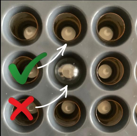
**3.** Preparing the capsule cap: Place the alignment plate on top of the cap plate. Repeat steps 2.2 – 2.3, now with the short part of the capsules filled into the alignment plate on top of the cap plate. When the process is complete, remove the alignment plate and set it aside.
