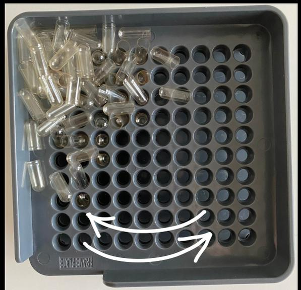
**2.3** Check that the capsules in the main board are located correctly. Where the capsules are upside down, change it to correct position.
