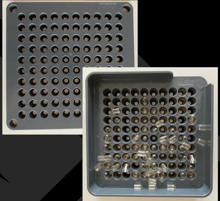
**4.** Filling the capsule body with powder: Take back the main board in which you have prepared the capsule bodies. Place a powder block on it and then add the powder on the board. Spread the granules evenly over the board by using spreader. Remove the excess granules.
