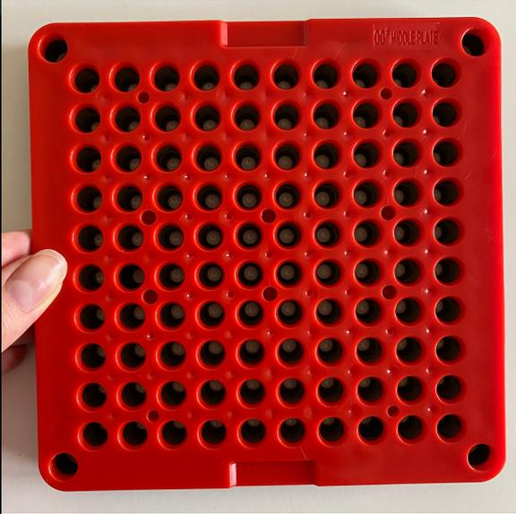
**6.2** Place the cap plate and middle plate on top of the main board as shown on figure below. Gently press down the plates.
