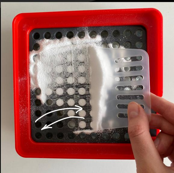
**5.** Compress granules by the tamper. Repeat step 4 and 5 a couple of times.
